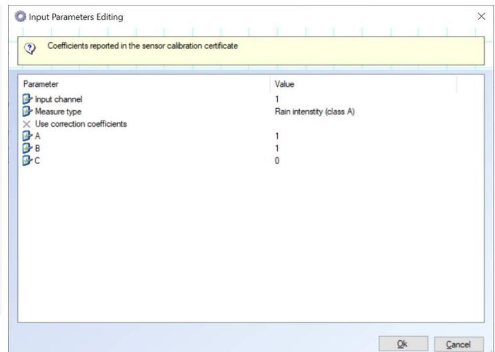
▶ Alpha-Log data logger has the corrective formula for precipitation intensities on board. Following the calibration procedure, parameters a, b and c are obtained to be inserted in the 3DOM configuration software. Thanks to this setting the values recorded by the data logger are already correct and have a relative residual error  $\leq \pm 3\%$  (Class A).
